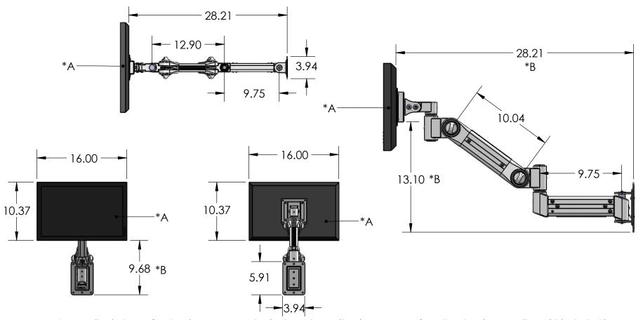
\*A: Monitor is shown for drawin purposes only. Customer's monitor size may vary from the drawing. Monitor NOT included in assembly \*B: Adjustable arm shown at 45 degrees. Arm can be adjusted from horizontal to vertical. Some dimensions may change as the arm moves
